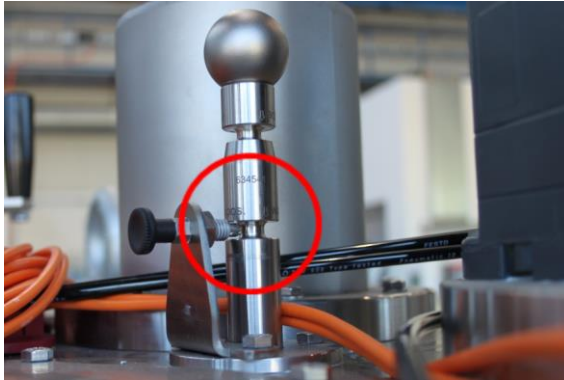
Fig. 114: Securing the rod in the "Production" position
