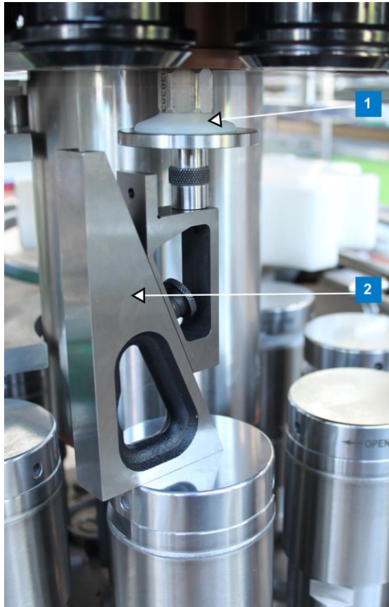
Fig. 110: Adjusting knock-out pad at the gauge
