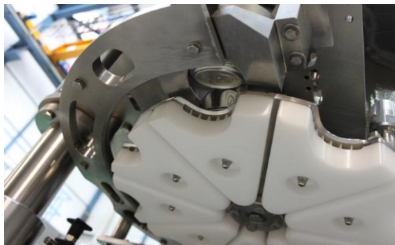
Fig. 118: Ends in the end feed magazine must be accessible from below
