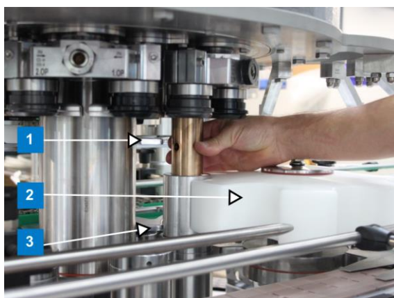
Fig. 53: Checking the discharge turret
